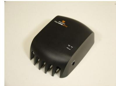
The FibreIRS GTU converts optical power to RF power (FM,DAB,DTT and 4 satellite polarities). The FibreIRS GTU has built in AGC which allows a wide dynamic range of optical powers without affecting output power and quality. Two LED indicators allow the user to observe the status of the unit.
